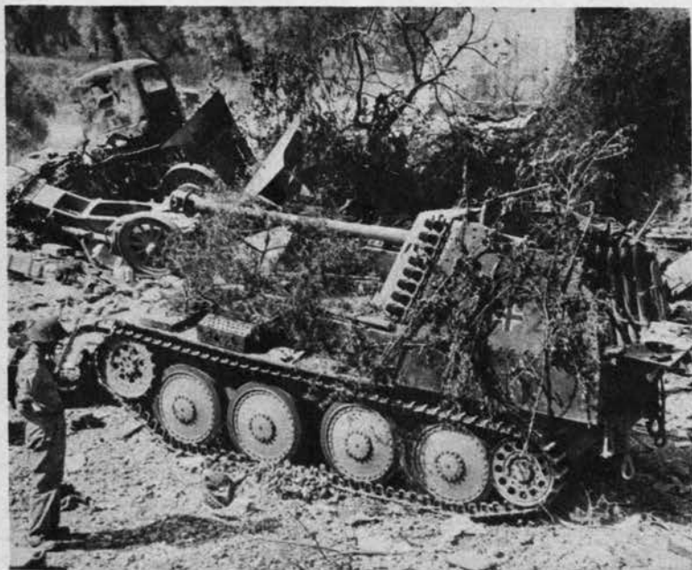
Slab-sided crew compartment of SP "75" is set far back. The Czech chassis has a short wheel base, four large Christie-type bogie wheels.
